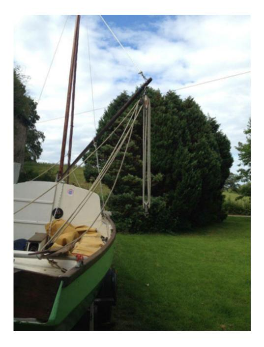
We set up the main halyard as the principle way to hold the boom in place and to be able to raise and lower it. I had taken off the boom anyway as I intend sailing her loose footed for now.
