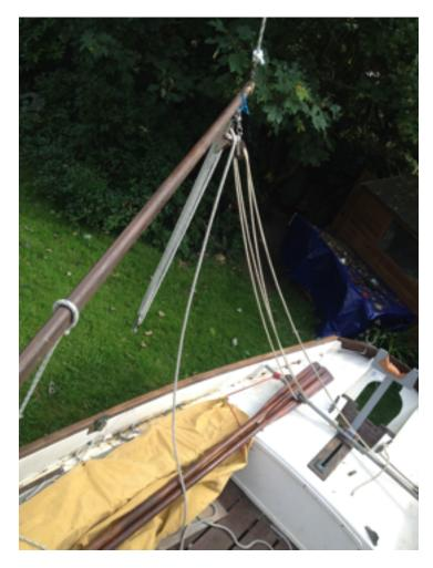
Now for testing; we put axle stands under the rear of the trailer and wood blocks under the end of the boats keel plank, to stop her tilting back, then attached a large bucket of water to the hoist to test its steadiness. We were a little concerned that the whole boat and trailer would tilt\*\*, but it didn't and allowed us to more easily lift the engine up and over the gunwales and then be swung across midships.
